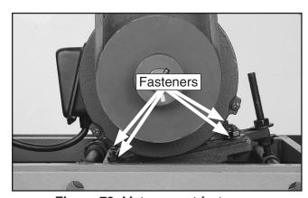
Figure 72. Motor mount fasteners.
